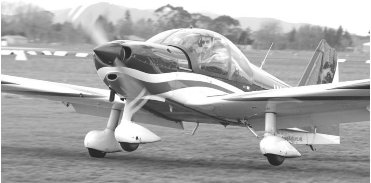
Figure Three - Landing Attitude for Low Wing Tri-Gear Aeroplane.
