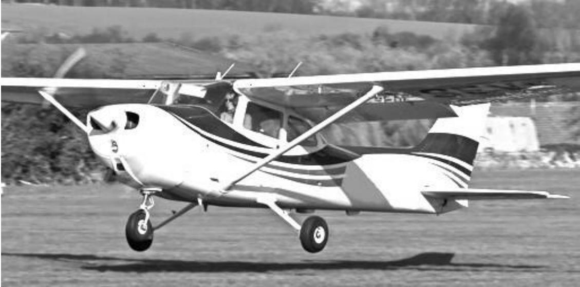
Figure Four - Landing Attitude for High Wing Tri-Gear Aeroplane.
