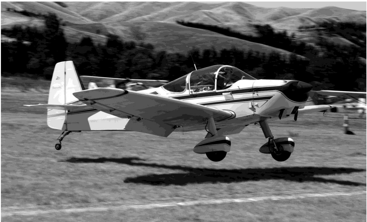
Figure Four. Tailwheel slightly below main wheels
