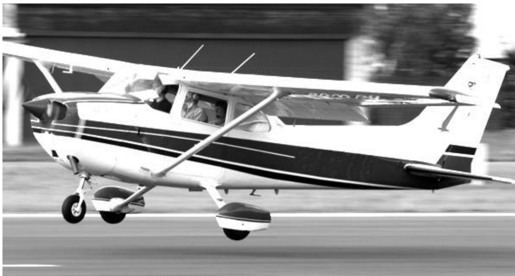
Figure Eight – Landing Attitude whilst Side Slipping in a Cross Wind
