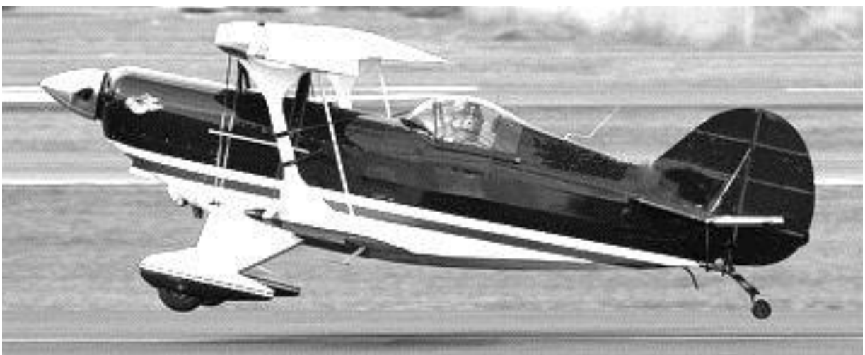
Figure Six – Pitts S2S in the 'Three Point' Attitude.
