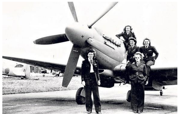
1945. Mk22 Spitfire: 1850HP, Five blade constant speed metal propeller.
