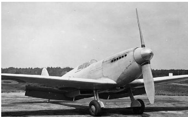
1936. Prototype Spitfire: 1050HP, Two blade fixed pitch wooden propeller.
