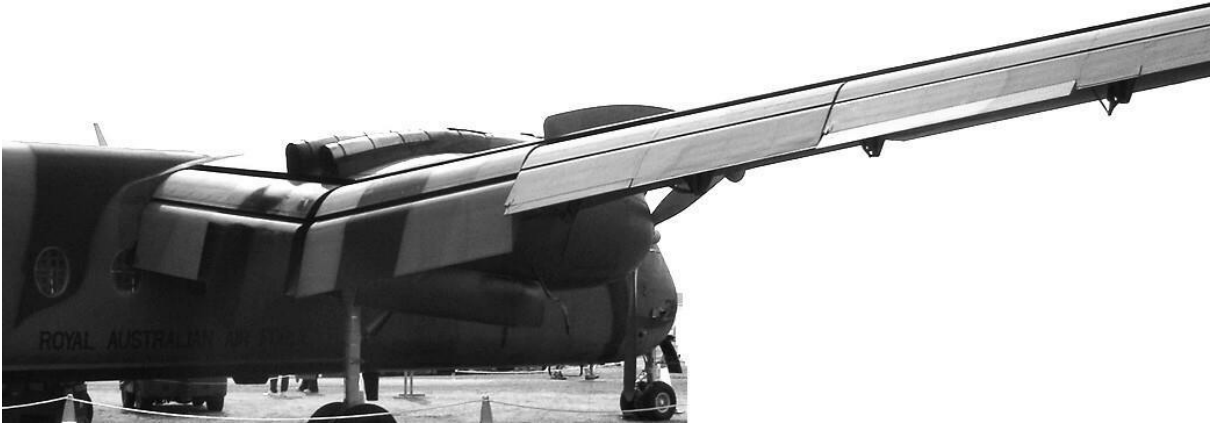
Figure Thirty Nine - Caribou full span double slotted flaps
