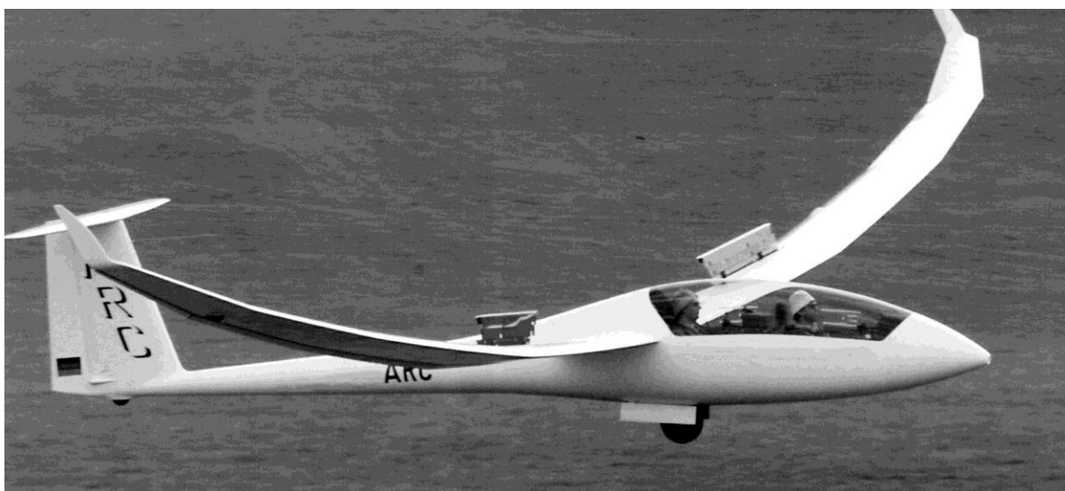
Figure Three – Wing ‘Bending’ exacerbated by use of Air Brakes
